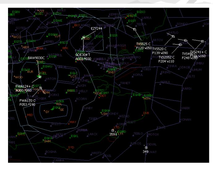
Synthetic image based on antenna angle, signal delay, squawk and altitude.
